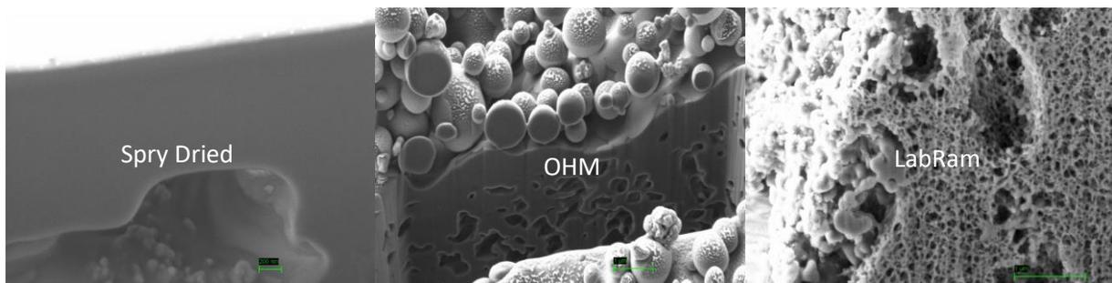
Figure 2. High magnification FIB-SEM cross section images.
