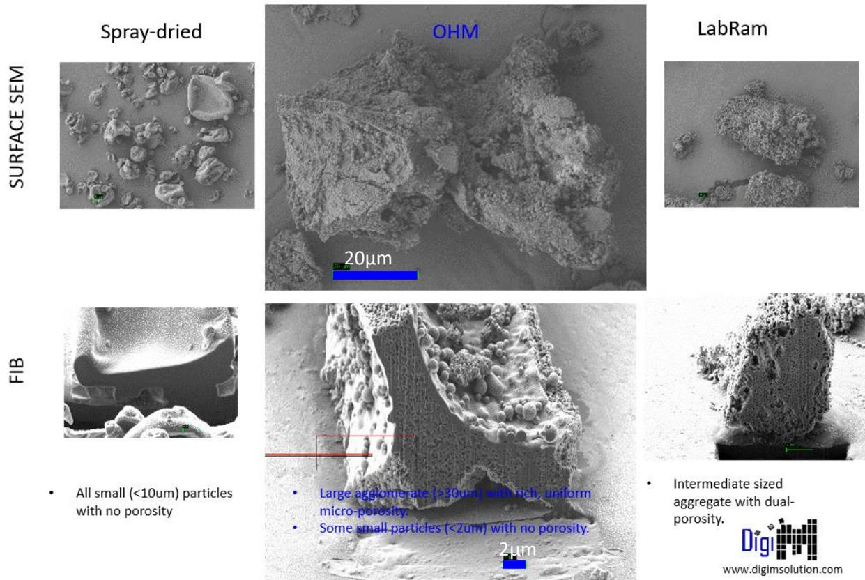
Figure 1. Comparison of sample external surface SEM overview at the same magnification, and the corresponding FIB cross section SEM at the same magnification (higher than the surface SEM magnification).
